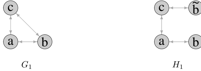
Figure 5: Node b is splitted by adding node \tilde{b} \notin \mathcal{V}_G to the network and replacing the edges in \{(b, c), (c, b)\} by those from \{(\tilde{b}, c), (c, \tilde{b})\} .
